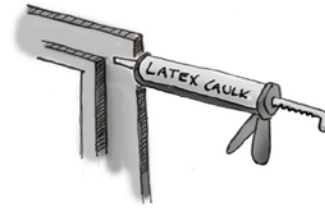
USE A GUN TO PUT CAULK INTO THE CORNERS LIKE THIS
