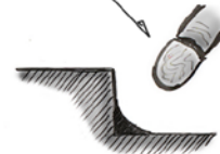
NEATLY APPLY THE CAULK WITH THE GUN BY TRIMMING THE SPOUT AT A SMALL ANGLE, AND USE PATIENCE SQUEEZING IT INTO THE CORNERS
